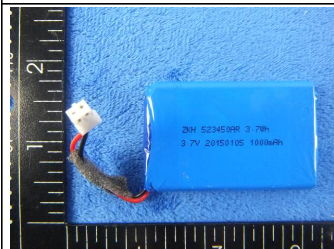
Battery - Rear View
