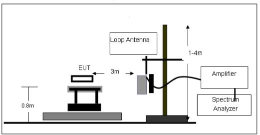
(B) Radiated Emission Test-Up Frequency 30MHz~1GHz
