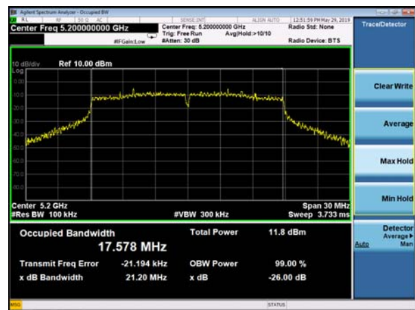
(802.11 n20) -26dB&99%Bandwidth plot on channel 48
