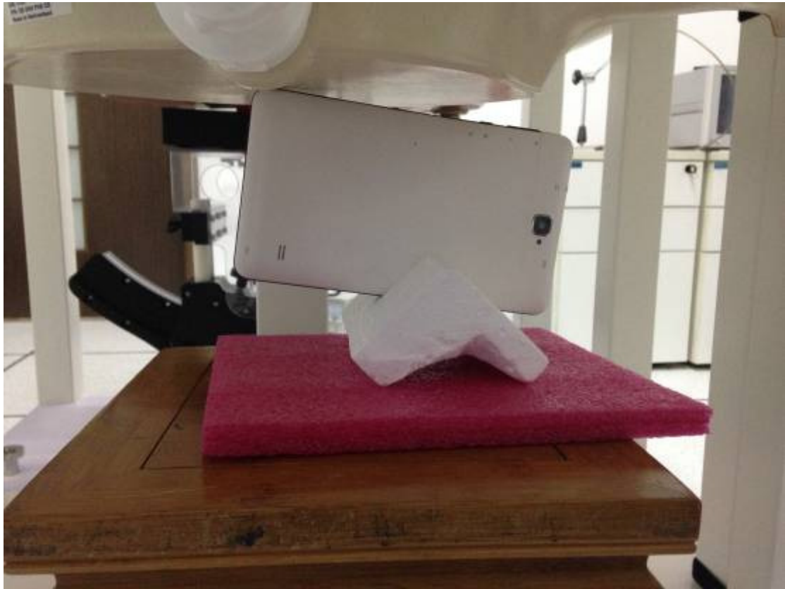
Body Bottom Edge/Right Corner with Right 40° Angel Tilted
