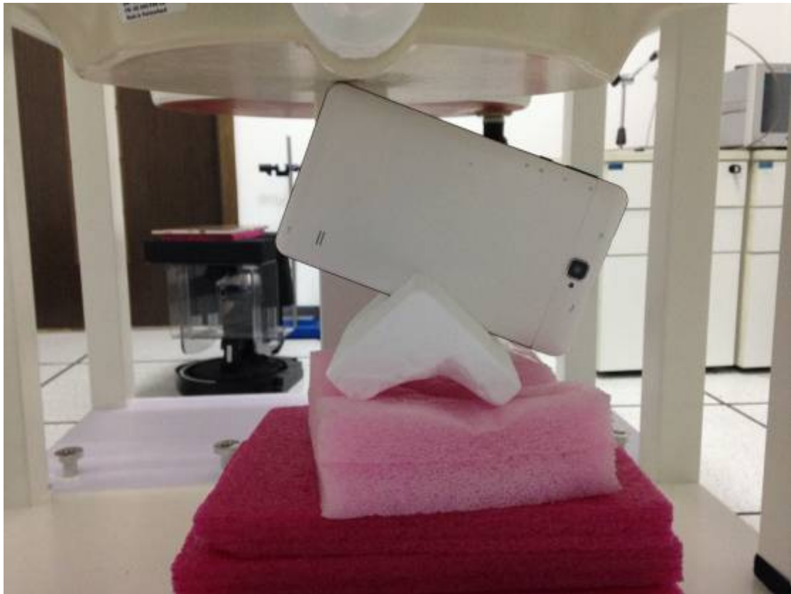
Body Bottom Edge/Right Corner with Right 30° Angel Tilted
