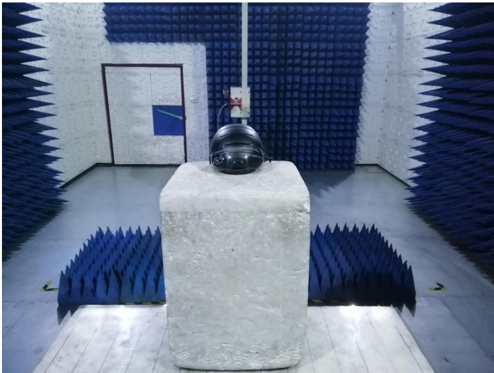
RADIATED EMISSION TEST SETUP ABOVE 1GHz
