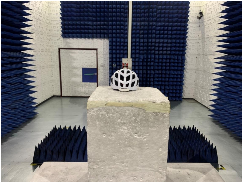
RADIATED EMISSION TEST SETUP ABOVE 1GHZ
