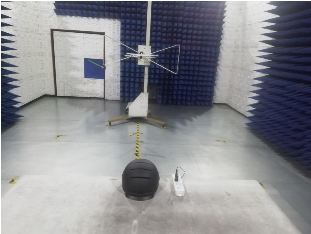
RADIATED EMISSION TEST SETUP ABOVE 1GHZ
