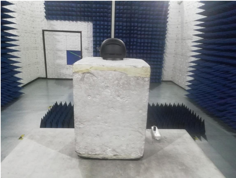
RADIATED EMISSION TEST SETUP ABOVE 1GHZ
