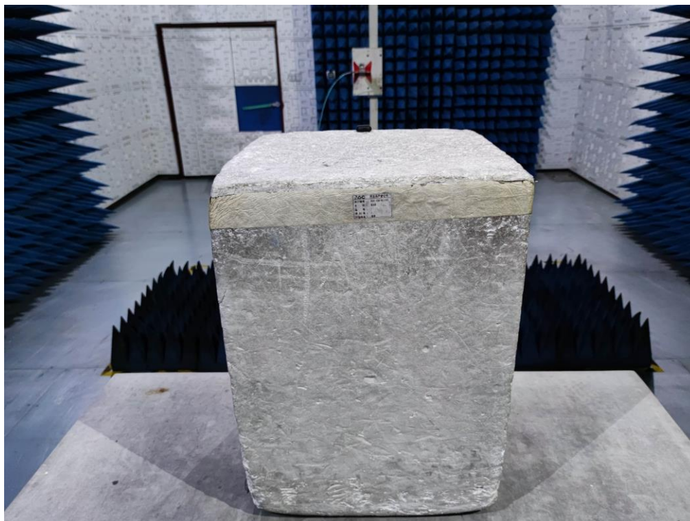
RADIATED EMISSION TEST SETUP ABOVE 1GHz
