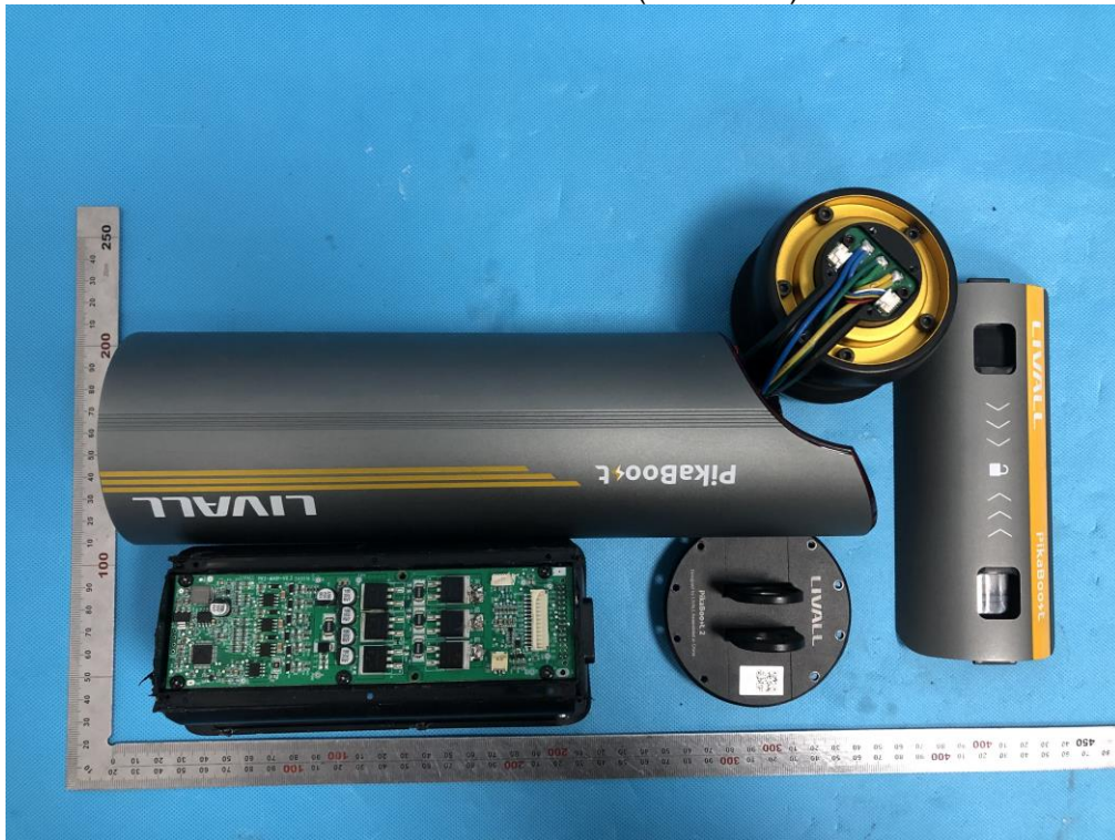
INTERNAL VIEW OF EUT (FIGURE 1)
