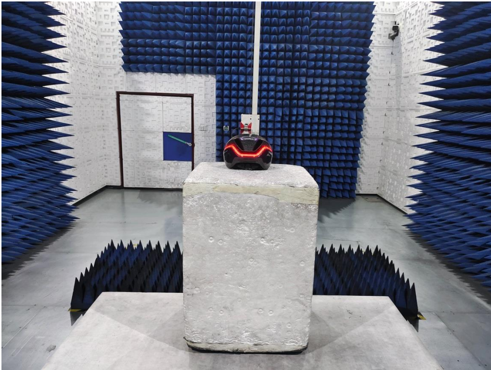
RADIATED EMISSION TEST SETUP ABOVE 1GHZ
