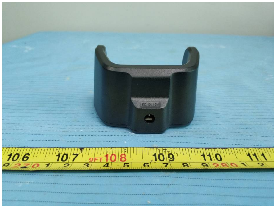
EUT – Charger Rear View
