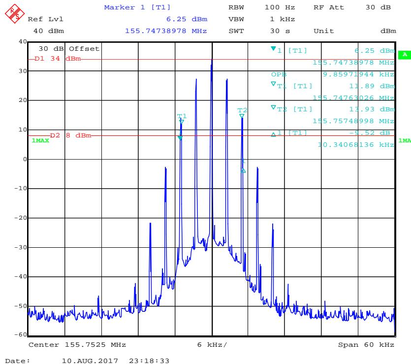
**Frequency 155.7525 MHz: 99% Occupied & 26 dB Bandwidth, Low Power**
