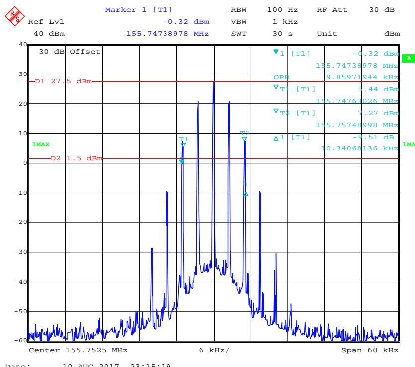
**Frequency 155.7525 MHz: Emission Mask, High Power**
