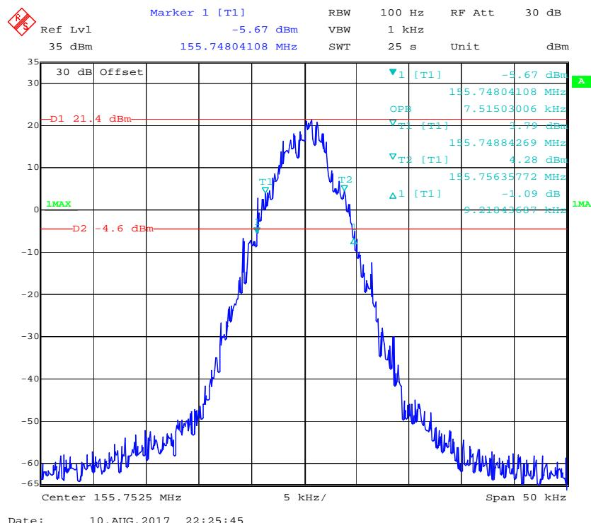
**Frequency 155.7525 MHz: Emission Mask, High Power**
