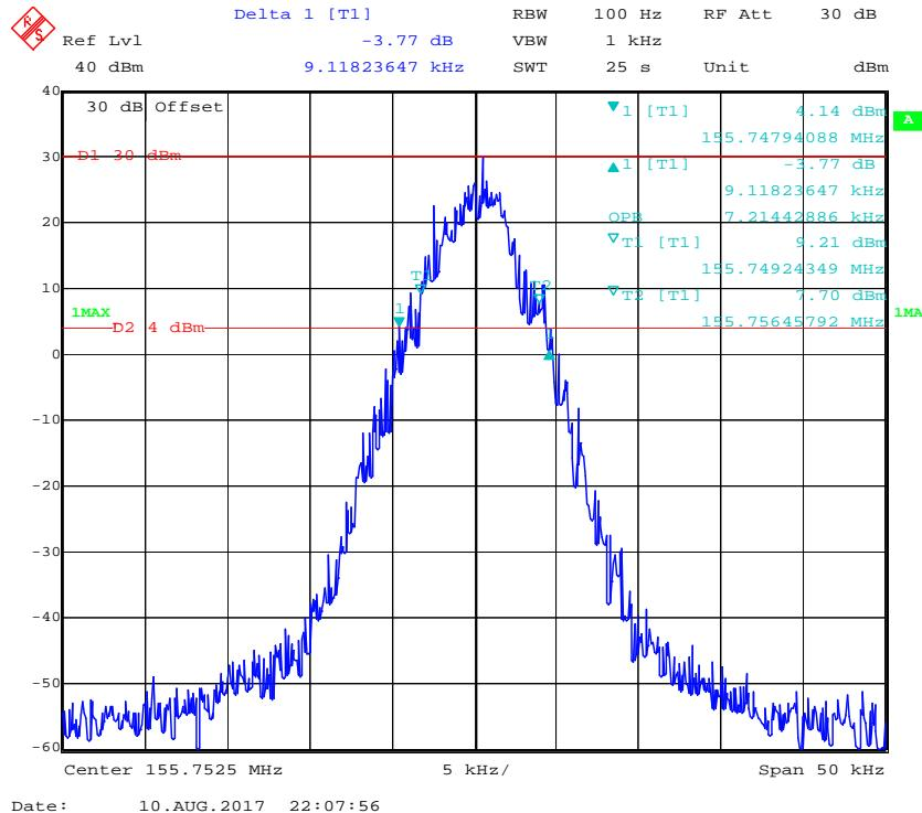
**Frequency 155.7525 MHz: 99% Occupied & 26 dB Bandwidth, Low Power**
