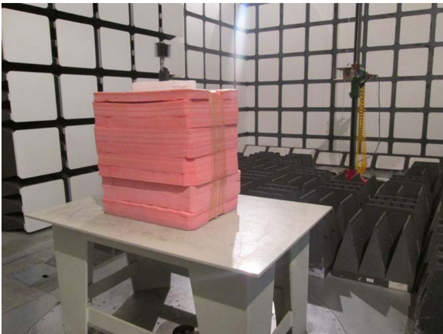
Transmitting Radiated Emissions View (Above 1 GHz)
