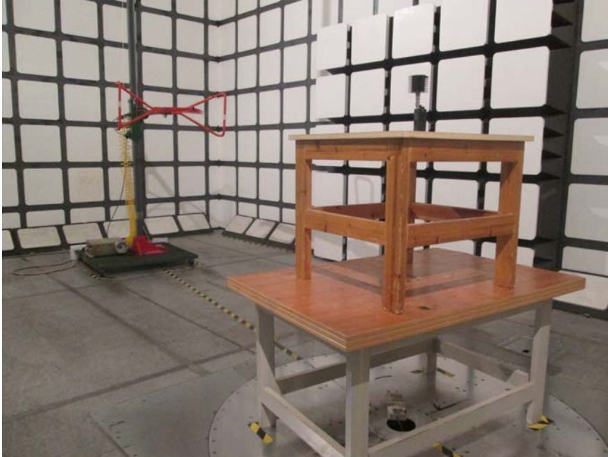
Transmitting Radiated Emissions View (Below 1 GHz)
