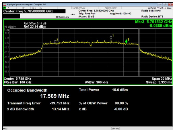
(802.11ac20) 6dB Bandwidth plot on channel 165
