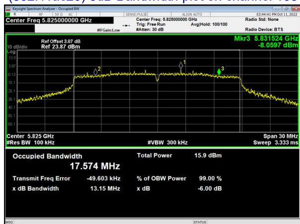
(802.11ac20) 6dB Bandwidth plot on channel 165
