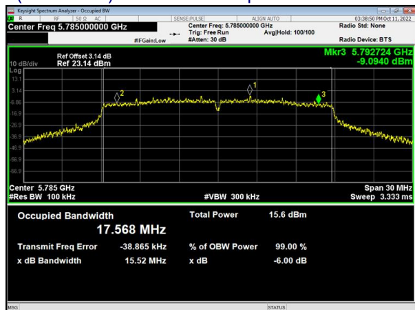
(802.11n20) 6dB Bandwidth plot on channel 157
