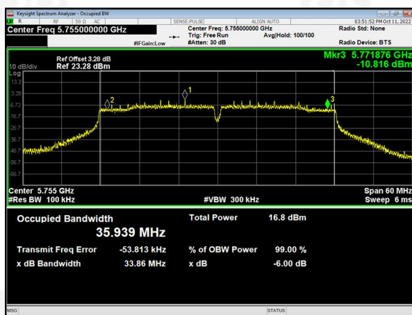
(802.11 ac40) 6dB Bandwidth plot on channel 159
