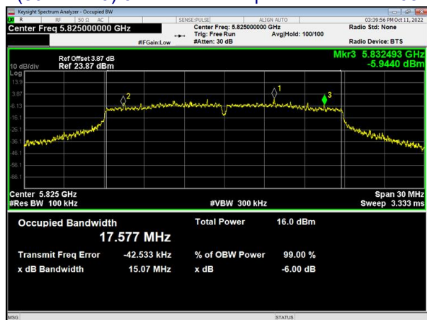
(802.11n20) 6dB Bandwidth plot on channel 165
