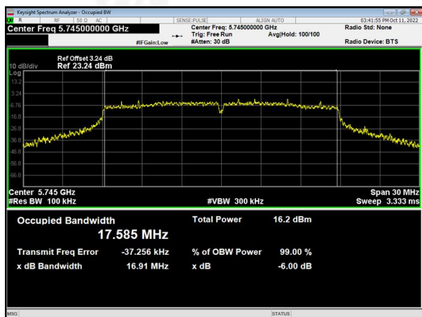
(802.11ac20) 6dB Bandwidth plot on channel 157
