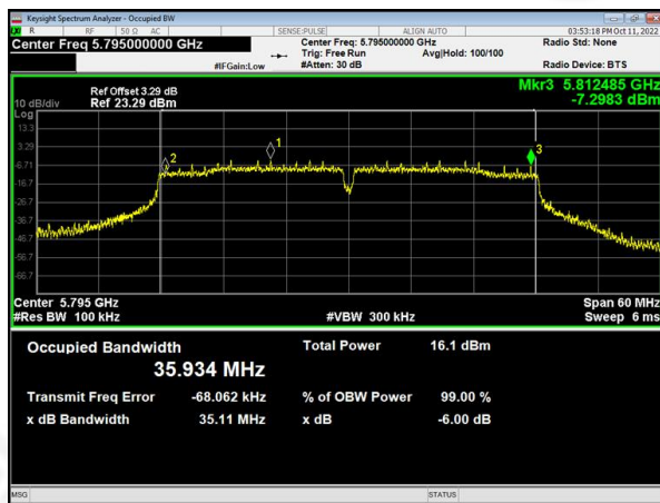
(802.11 ac40) 6dB Bandwidth plot on channel 159
