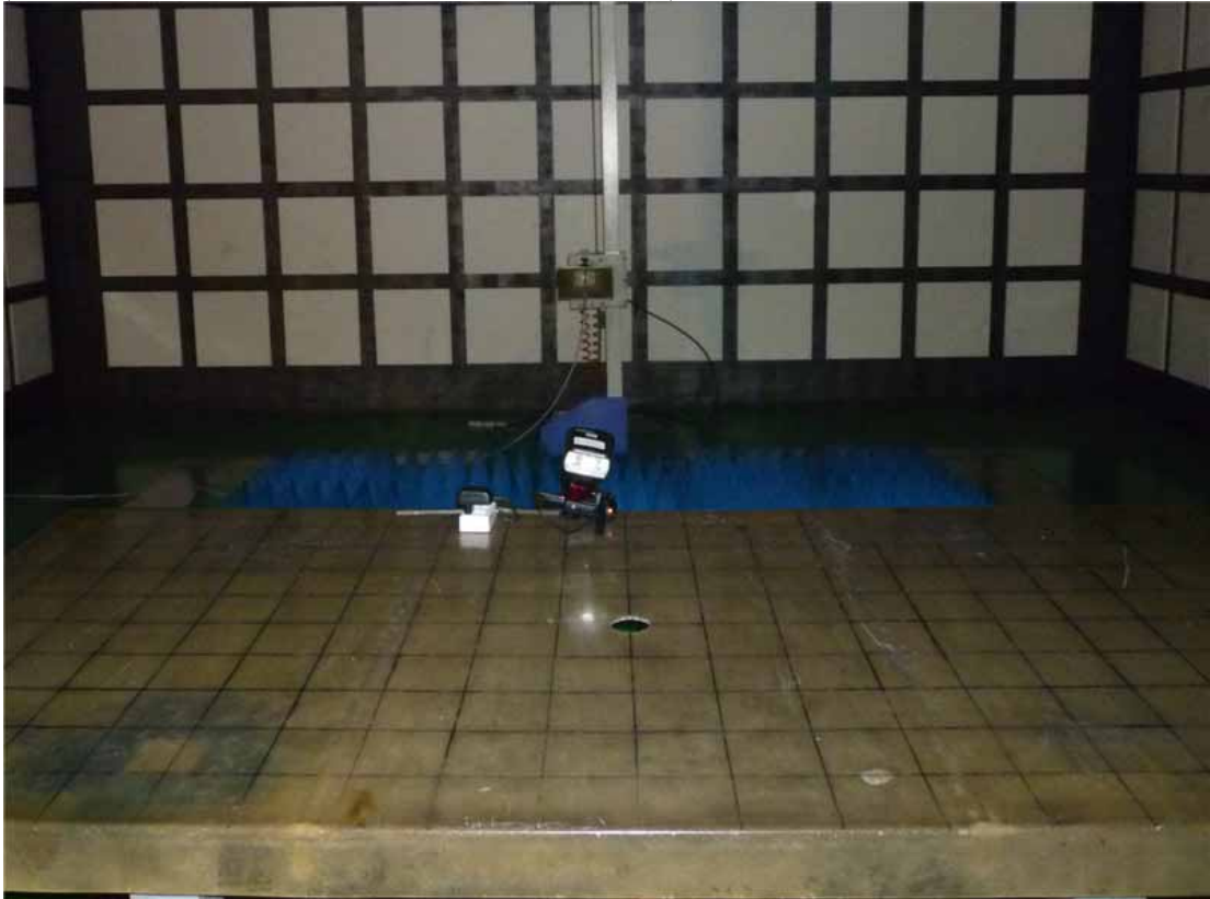
(At Anechoic 3m Chamber Test 1GHz –18GHz)
