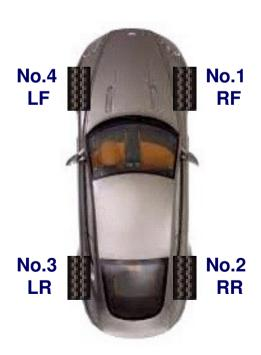
a. Put CR1632 battery into the No.1 (RF) transmitter.
