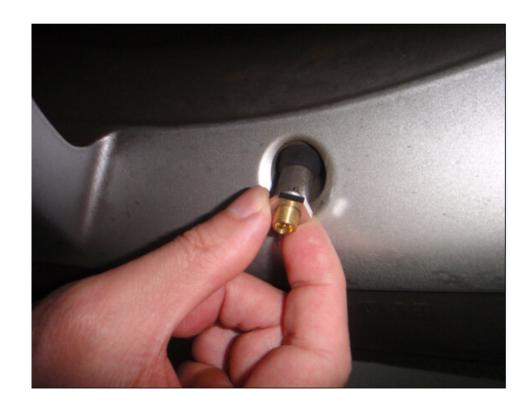
d. Lock No.1 transmitter to the right front tire valve and tighten it.
