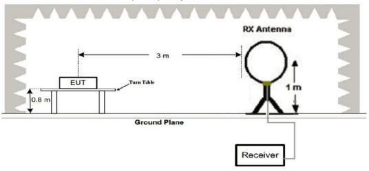
(1) Radiated Emission Test-Up Frequency Below 30MHz
