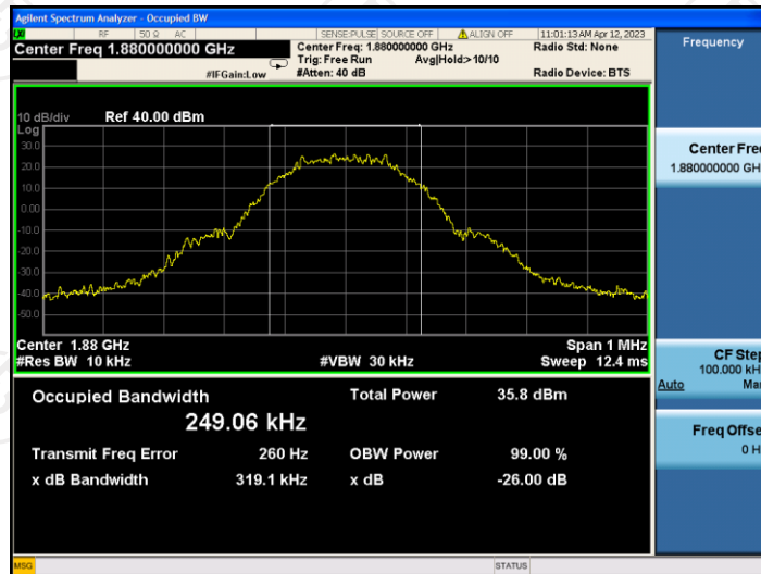
26dB&99% Occupied Bandwidth Plot on Channel 810
