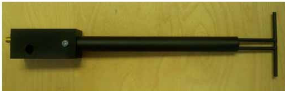
Figure 1 – MVG COMOSAR Validation Dipole
