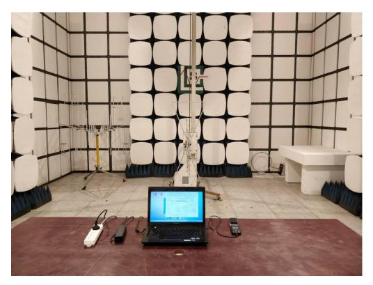
Test Setup Photo of Radiated Measurement (30MHz~1GHz)
