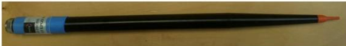
Figure 1 – MVG COMOSAR Dosimetric E field Dipole
