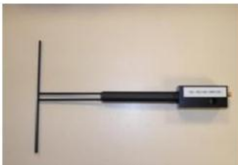
Figure 1 – Satimo COMOSAR Validation Dipole
