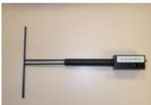
Figure 1 – Satimo COMOSAR Validation Dipole
