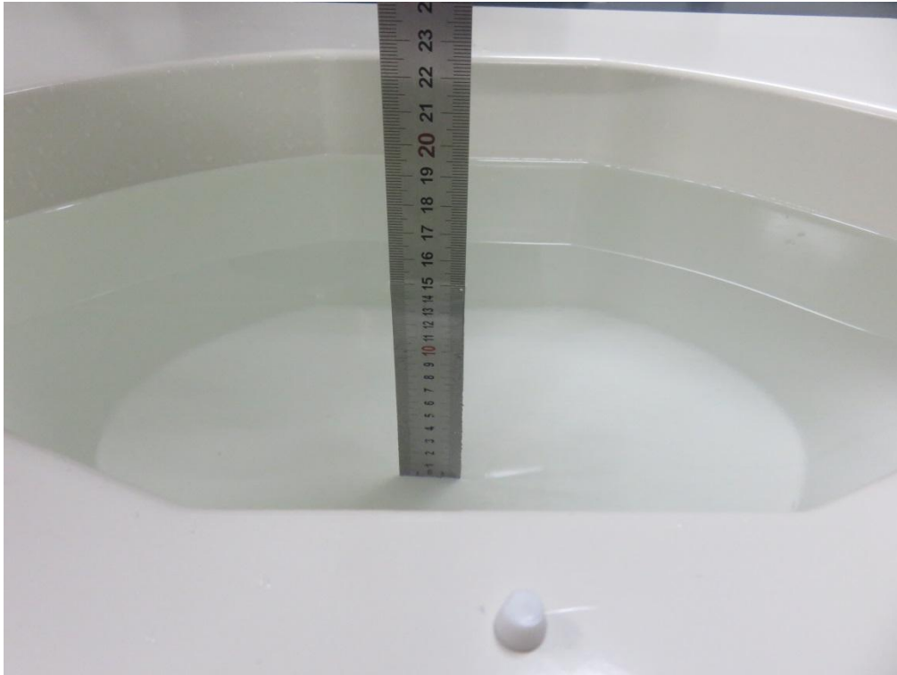
Photograph of the depth in the Body Phantom (835MHz, 15.1cm depth)
