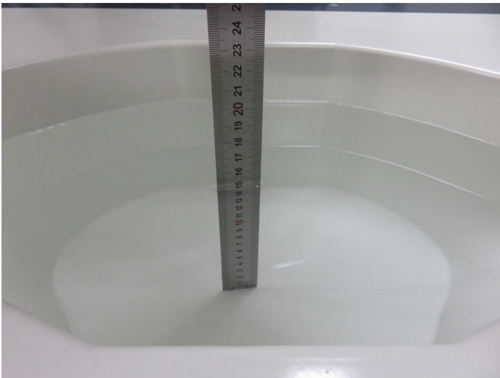
Photograph of the depth in the Body Phantom (1900MHz, 15.2cm depth)
