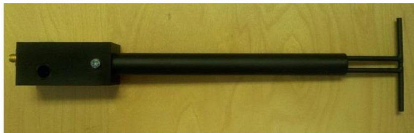
Figure 1 – MVG COMOSAR Validation Dipole
