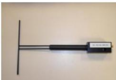
Figure 1 – Satimo COMOSAR Validation Dipole
