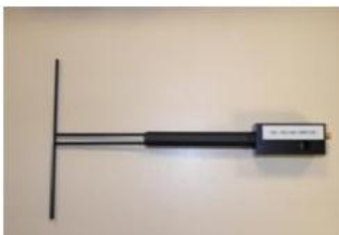
Figure 1 – Satimo COMOSAR Validation Dipole
