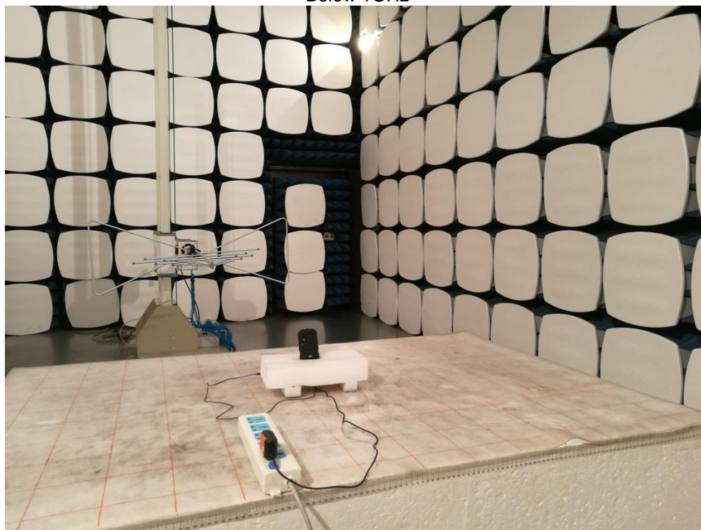
Radiated Spurious Emission Below 1GHz
