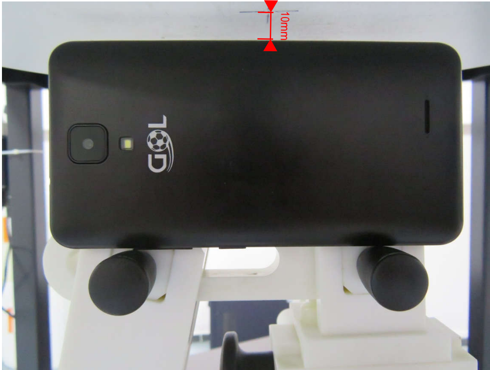
10mm body-worn Left Side Setup Photo(hotspot)
