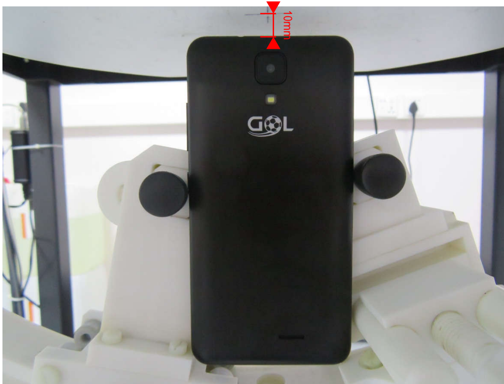
10mm body-worn Top Side Setup Photo (hotspot)
