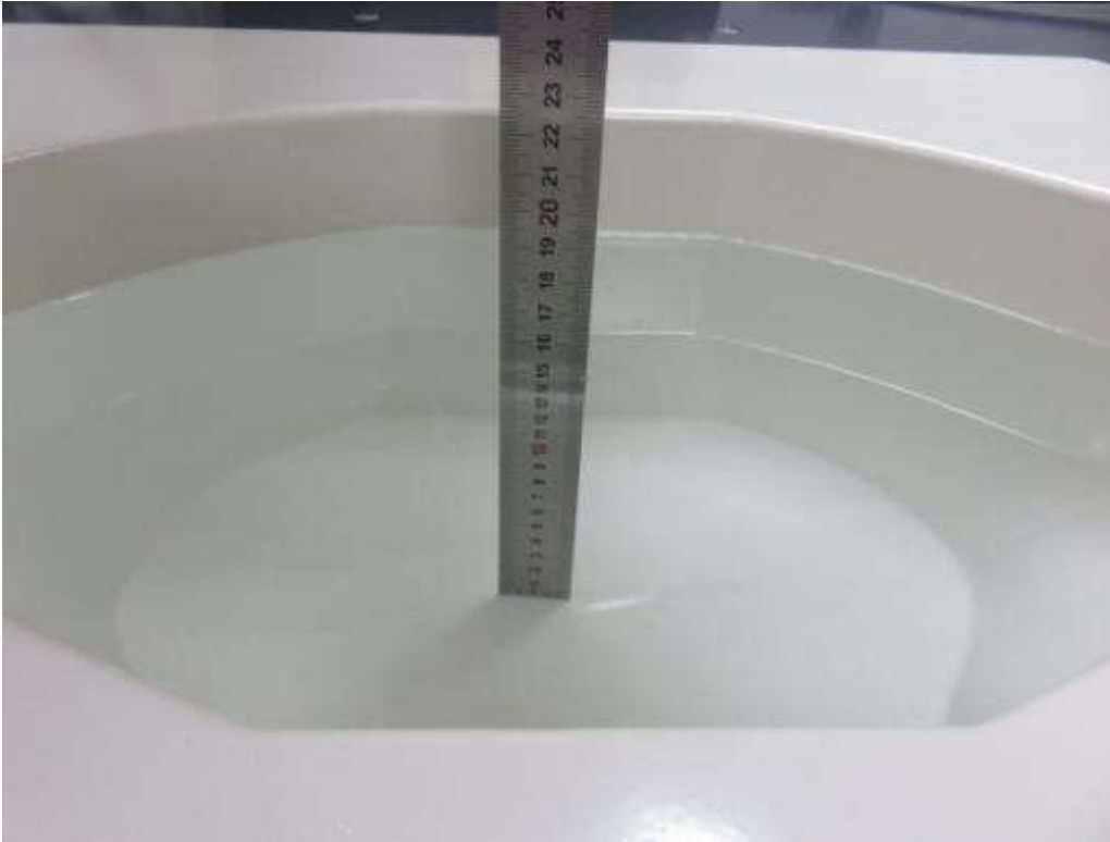
Photograph of the depth in the Body Phantom (1800MHz, 16.0cm depth)
