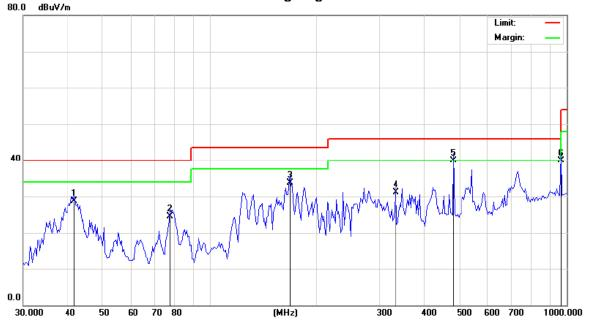
Limit: FCC Part 15B Class B RE 3 m Mode: Charging and DATA Transmtting
