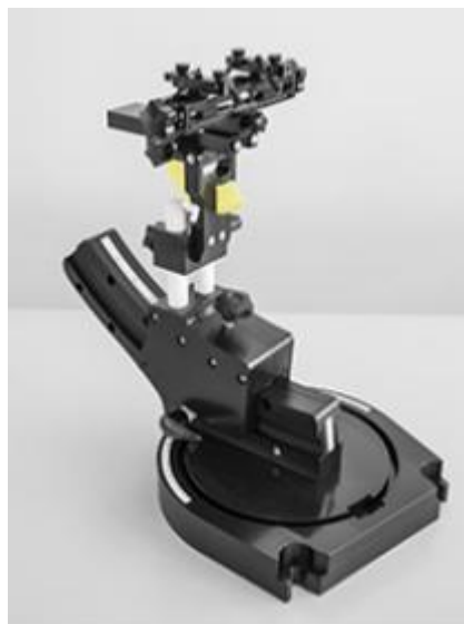
Device holder supplied by SPEAG
