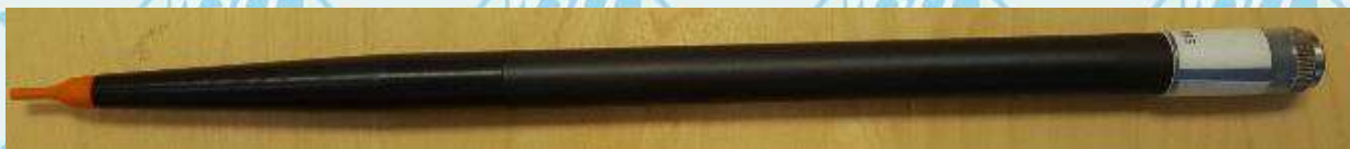
Figure 2 – MVG COMOSAR Dosimetric E field Dipole
