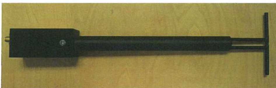
Figure 1 – MVG COMOSAR Validation Dipole
