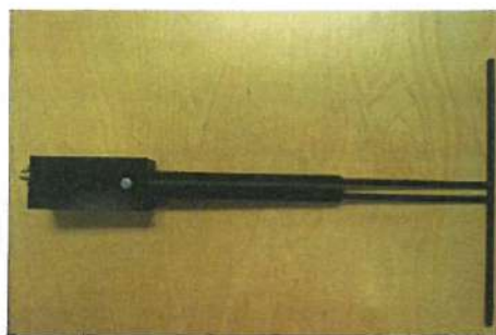
Figure 1 – MVG COMOSAR Validation Dipole
