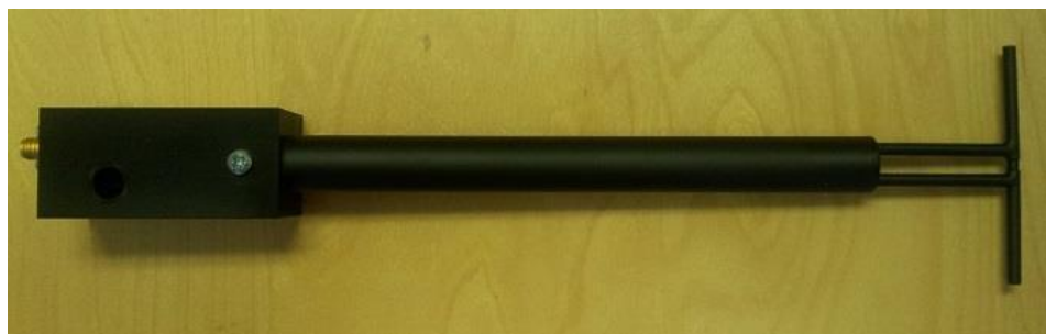
Figure 1 – MVG COMOSAR Validation Dipole
