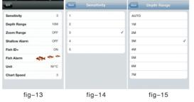
1) Sensitivity: Sensitivity is set as 1-5; this option is used to adjust the sensitivity of the sonar, as shown in Figure 14.
