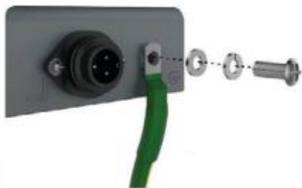
Connect Ground Cable at Rear Side
