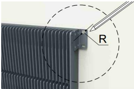
Marking the Position of Mounting Holes
