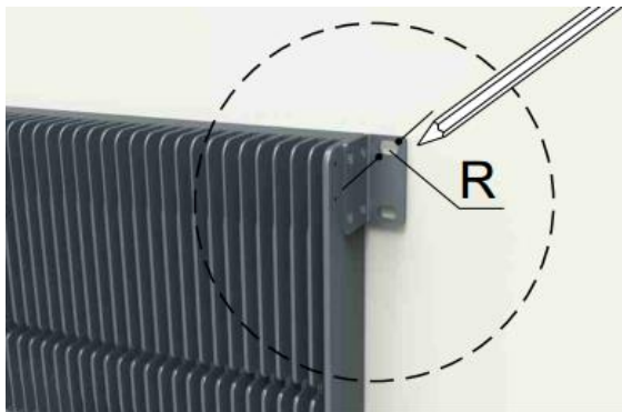
Marking the Position of Mounting Holes
