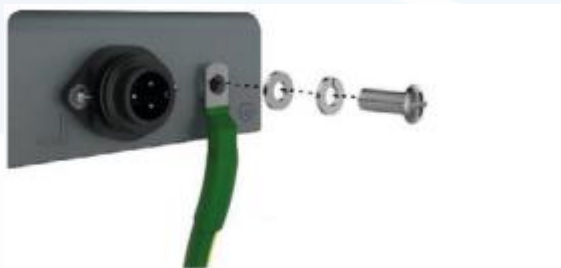
Connect Ground Cable at Rear Side
