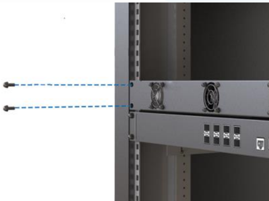
Fix Fan with Screws
