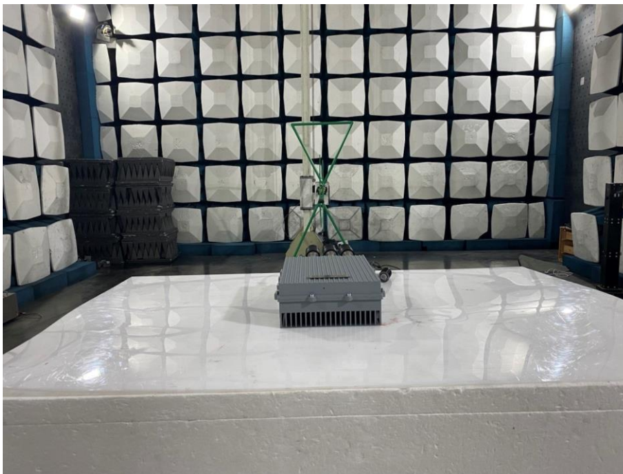
Radiated Emission Test Setup (Below 1GHz)
