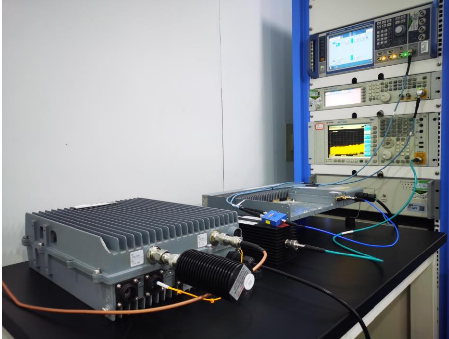
RF conducted test setup
