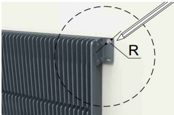
Marking the Position of Mounting Holes
