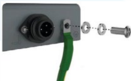
Connect Ground Cable at Rear Side
