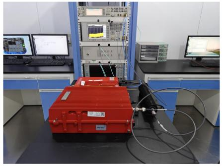
Radiated Spurious Emissions (30MHz-1GHz)
