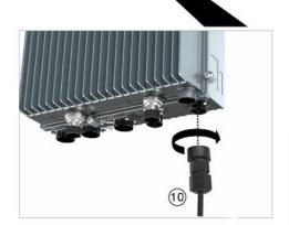
Connect and tighten the power cable to MP-PS.
