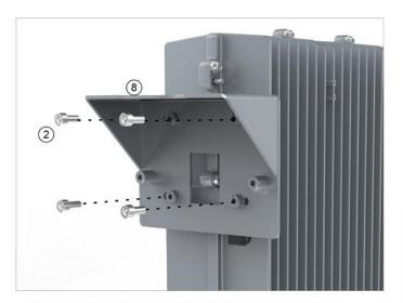
Fasten the mounting bracket I to the back of MP-PS with  $4\times M16\times 14$  screws.
