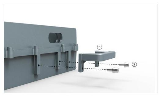
Fasten the handle to the side of MP-PS with 2×M6×14 screws.
