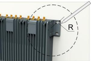
Mark 4ר6.8 holes sites for the hanger to be attached to the wall.
