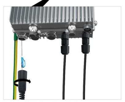
Connect and tighten the waterproof cable (\( \rightarrow waterproof sleeve to be purchased separately \)) to MP-PS.
