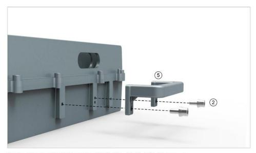
Fasten the handle to the side of MP-PS with  $2 \times M6 \times 14$  screws.
