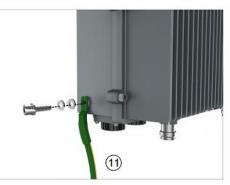
Connect and screw the ground wire to MP-PS.
