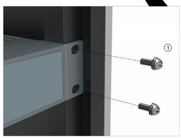
Install the AU-PS into the 19" rack and fasten with 4×M6 screws.
