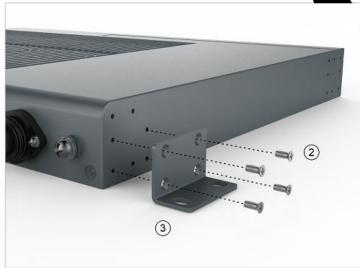
Rotate the hanger 90° and install in AU-PS.
