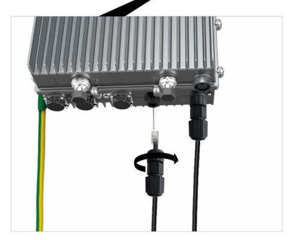
Connect and tighten the waterproof cable ( waterproof sleeve to be purchased separately) to MP-PS.
