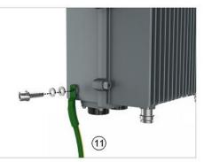
Connect and screw the ground wire to MP-PS.
