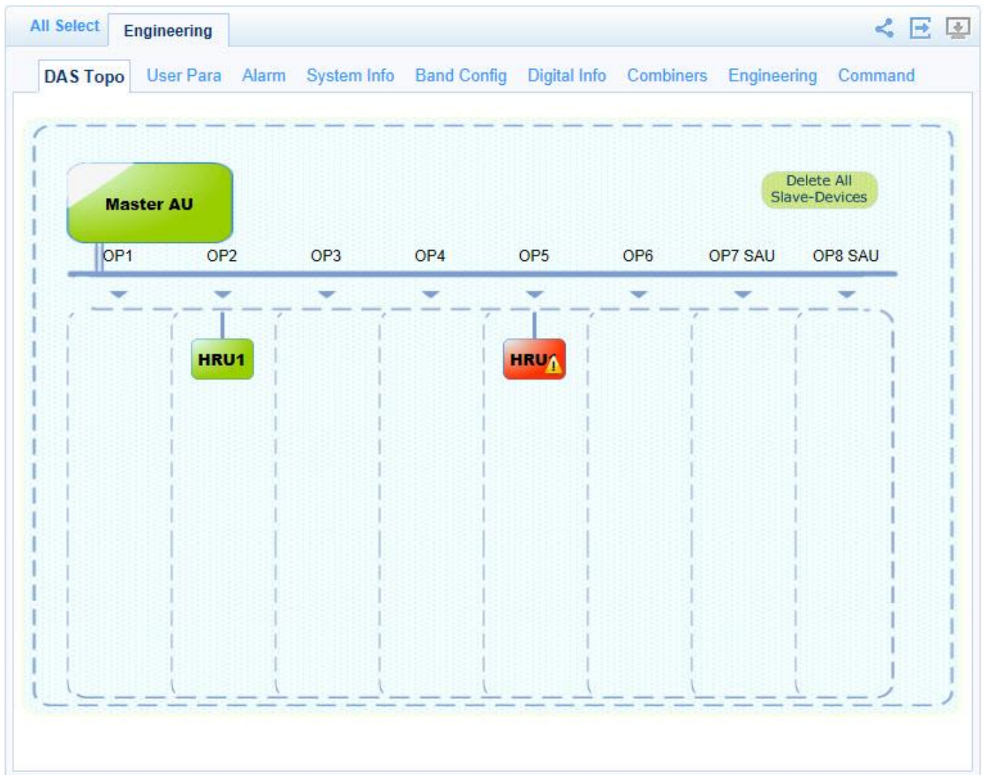
Figure 2-18 Displaying the System Topology
