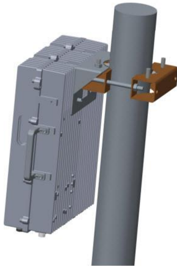
Figure 6-10 Schematic of RU Pall Installation
