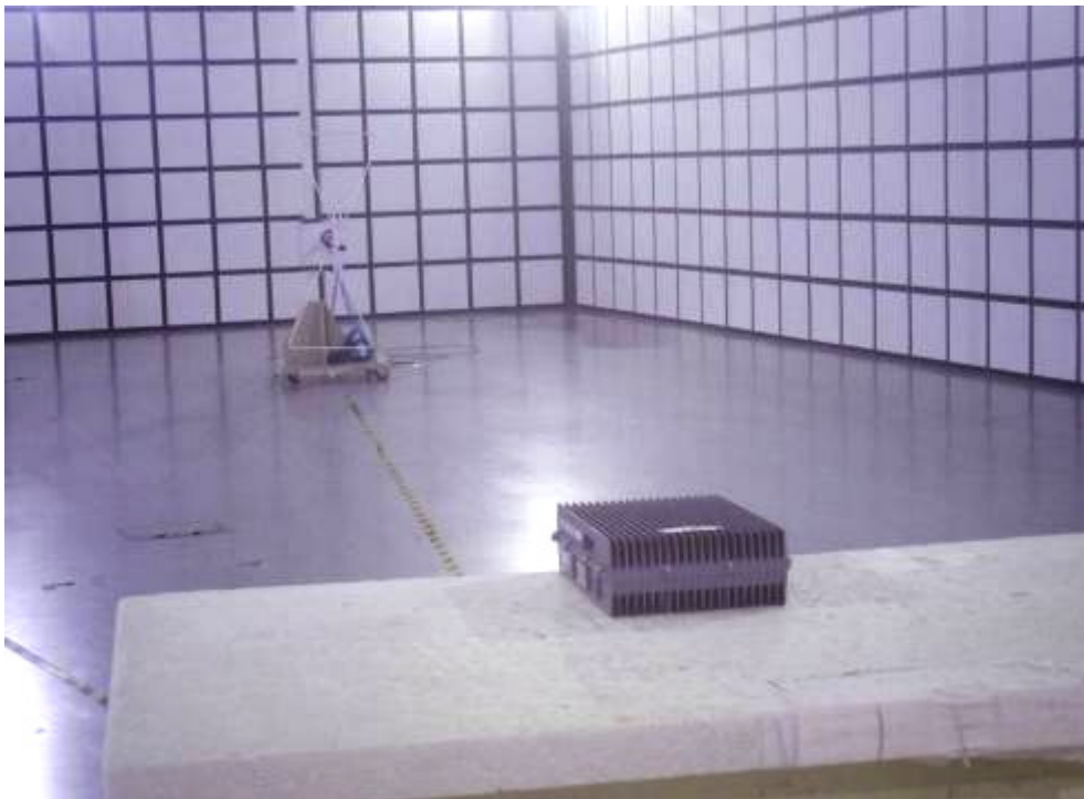
30MHz ~ 1GHz Radiated Emission
