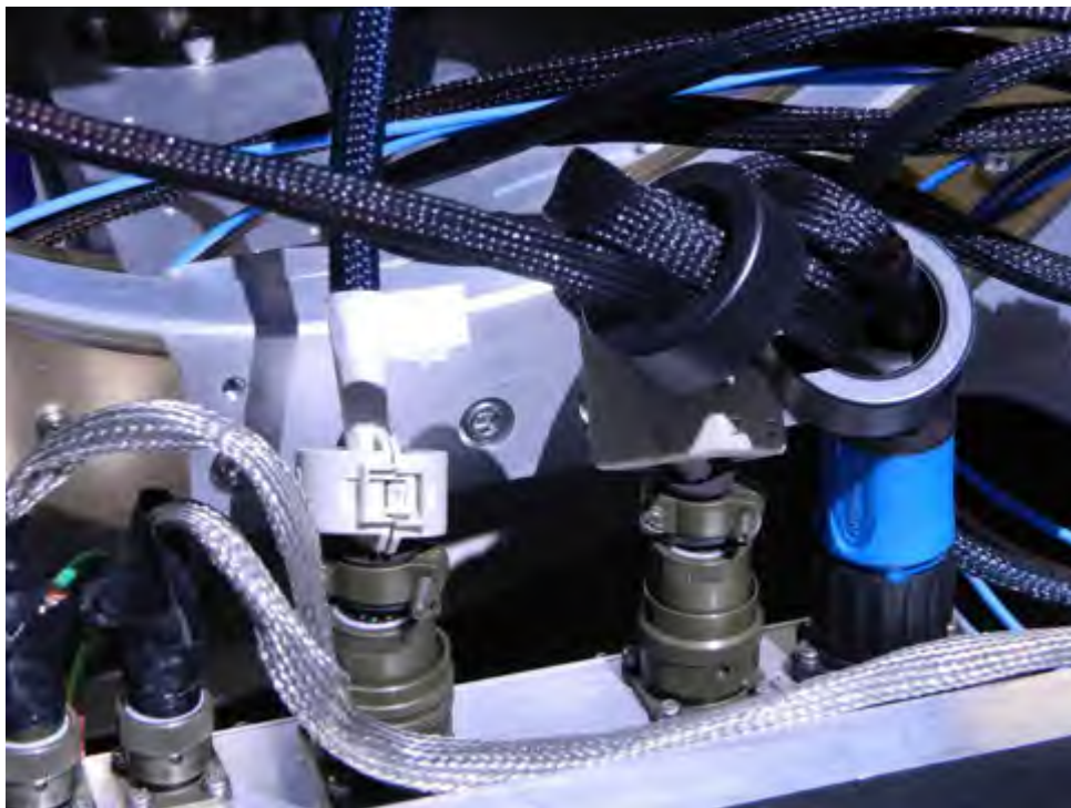
Photo 6 - Close up of ferrites on the cables, 1.2m dish
