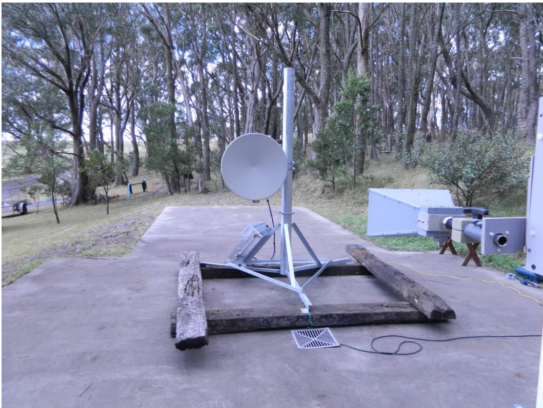
Photo 8 - EUT (0.6m dish) at the open area test site (OATS)
