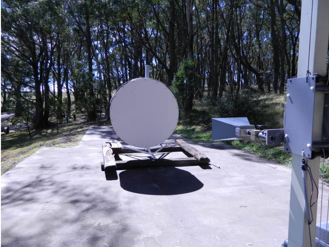
Photo 1 - EUT (1.2m dish) at the open area test site (OATS)
