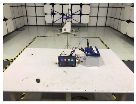
**Radiated Test (Above 1GHz)**
