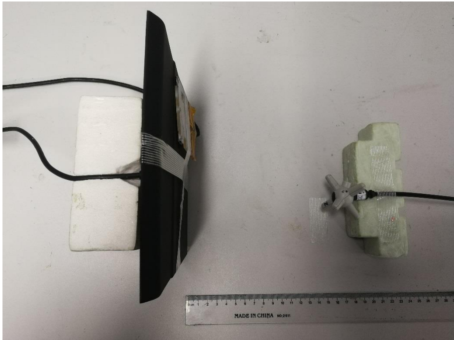
E-field Test Setup Photo Positon E Load1 (15cm)
