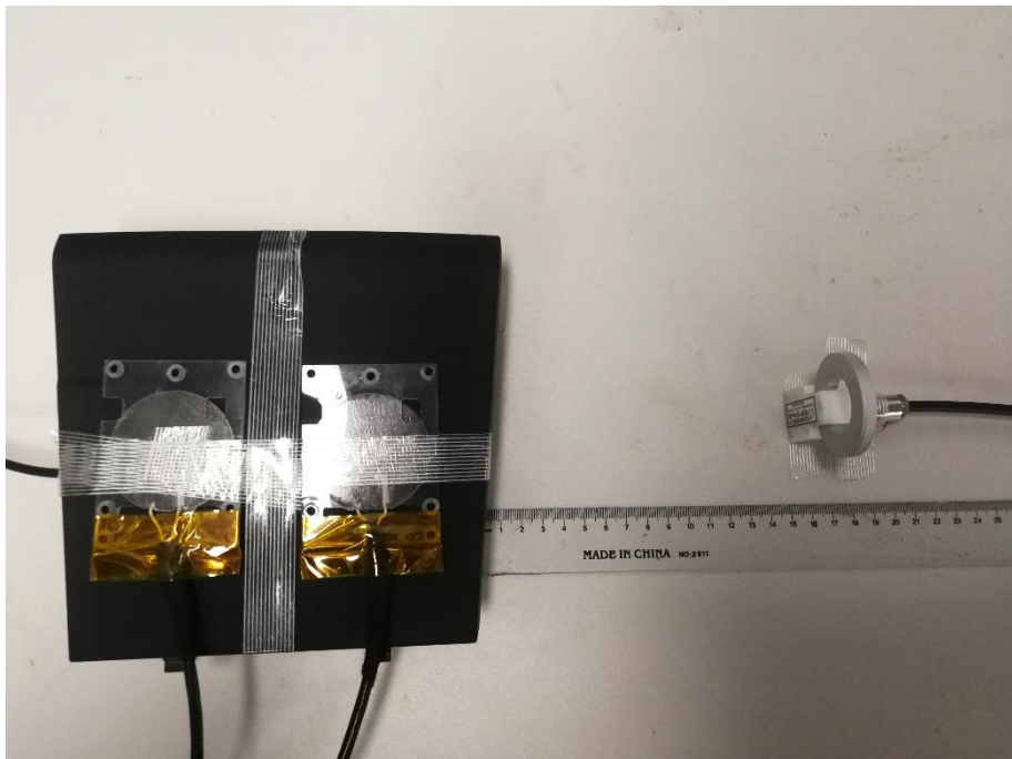
H-field Test Setup Photo Positon D Load2&3 (15cm)
