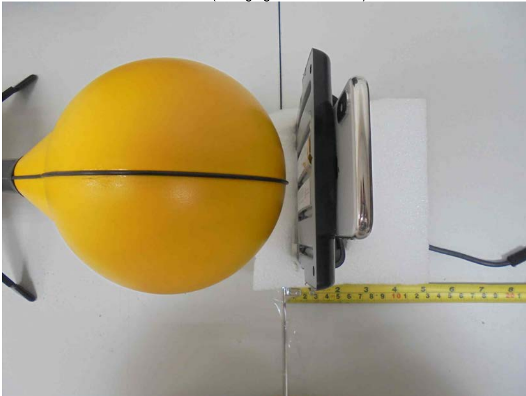
H-Field (Charging Mode - Bottom)
