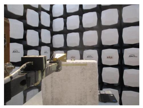
1.6 18 – 26.5 GHz at 1 Meter Rear View
