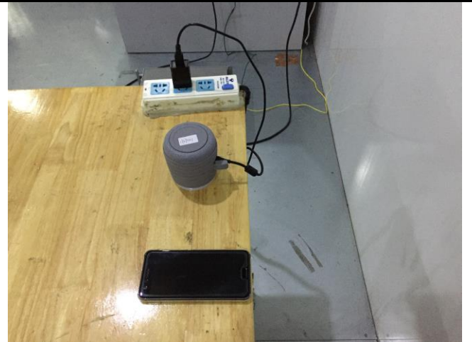
Conducted Emissions Test Setup Side View
