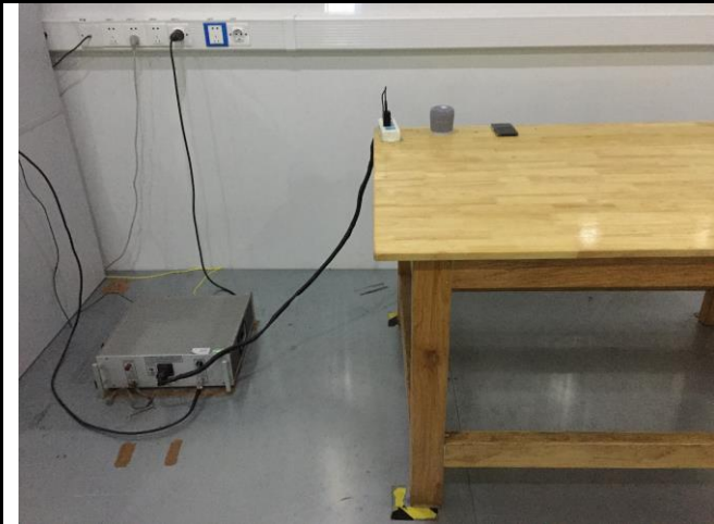
Conducted Emissions Test Setup Front View
