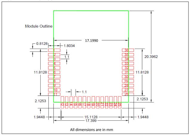
Module Keep-Out Area: - An area of 1.5mm around the module should be reversed as a keep-out area. No component should be placed in this area.
