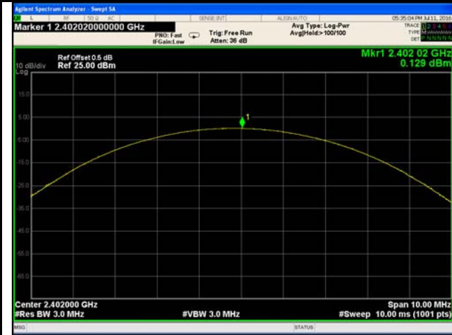
8DPSK Output power - Low CH 2402
